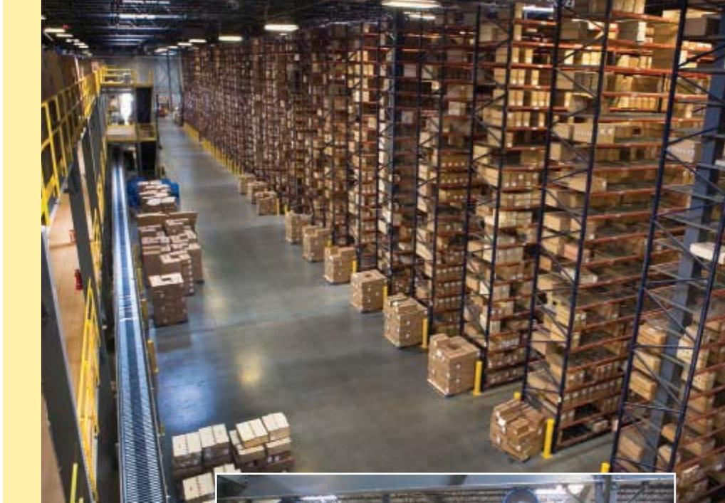
**After receiving (top photo), product is staged for putaway in racks. In the pick-to-light area (bottom photo), order selectors pick items that might be spread across multiple orders.**
