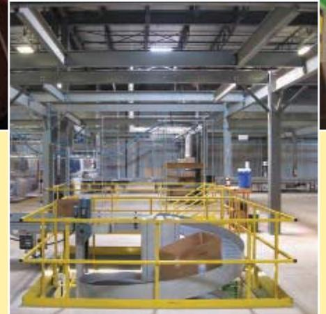
The Apparel Group's new DC brought together several materials handling automation technologies, including roller and spiral conveyor, tilt tray sortation, pick-to-light and RF picking technologies and a garment-on-hanger rail system.
